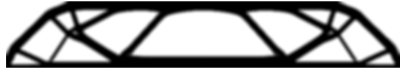
Figure 3. An optimized bridge structure at a resolution of 600 \times 100 with a distributed load around the center top quarters and constrained supports at the bottom corners. With higher resolution the optimization will place more fine struts.
