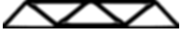
Figure 2. An optimized bridge structure at a resolution of 360 \times 60 with a single point load in the top center and constrained supports at the bottom corners. The optimization naturally tends towards to creating strut-like structures.
